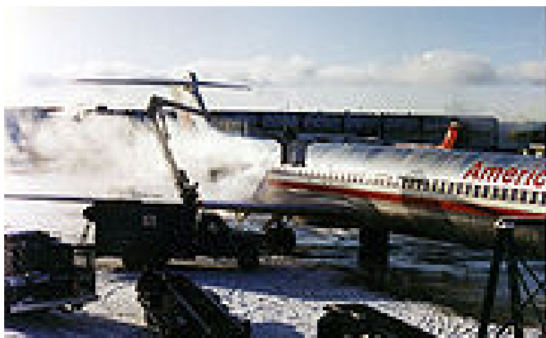
A de-icing vehicle treating an American Airlines MD-80 at Syracuse Hancock International Airport, New York
